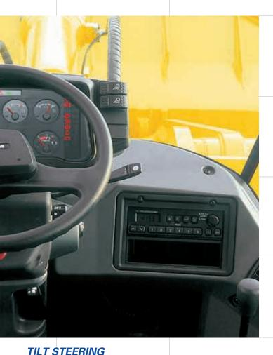
The tilt steering column adjusts to fit a variety of operator needs and offers greater comfort and efficiency.
